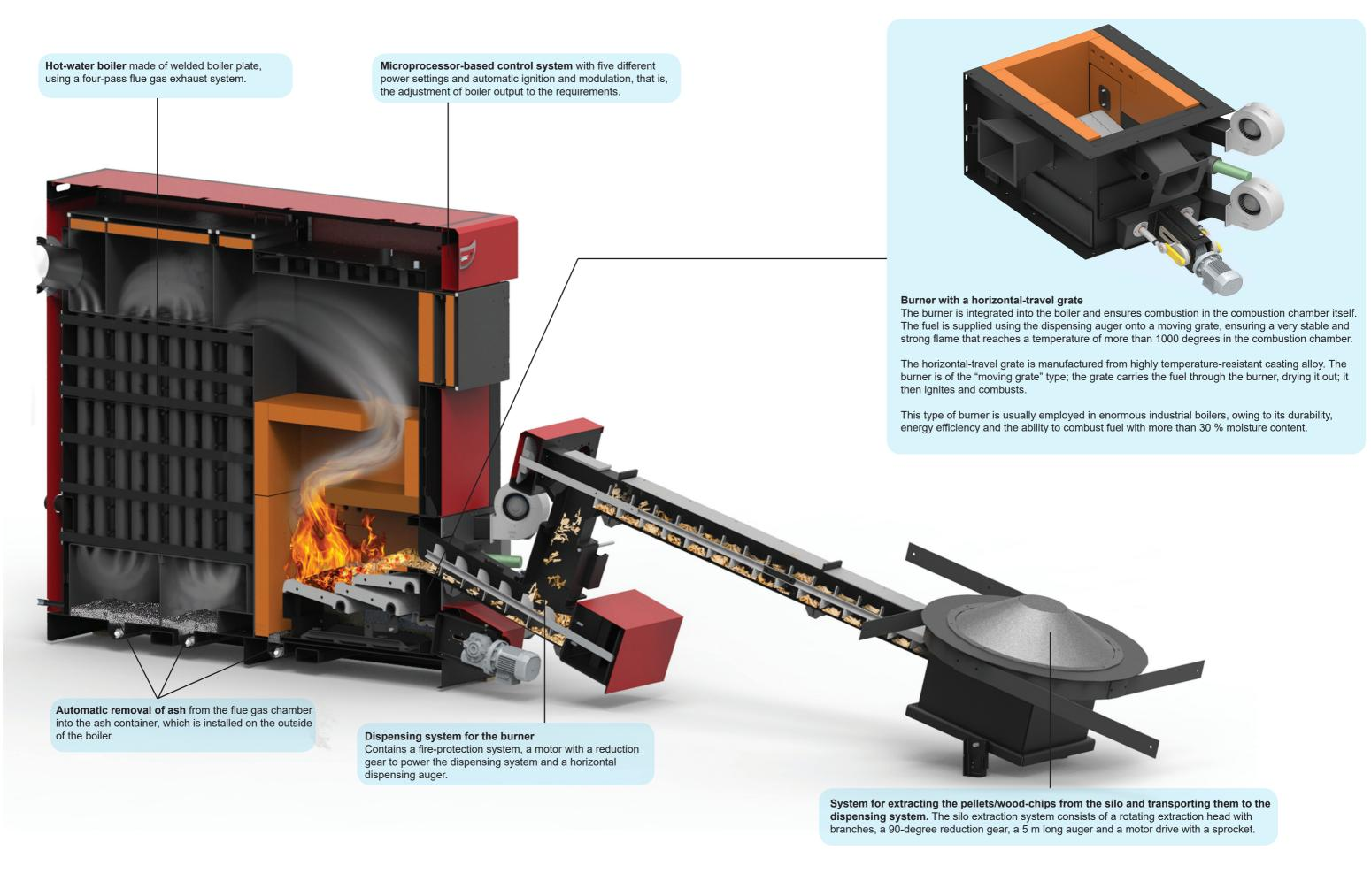
The system for supplying and dispensing pellets or wood-chips from the silo is suitable for places with sufficient space available on the outside. The extraction system is universal and can be integrated into silos of various shapes and sizes.
